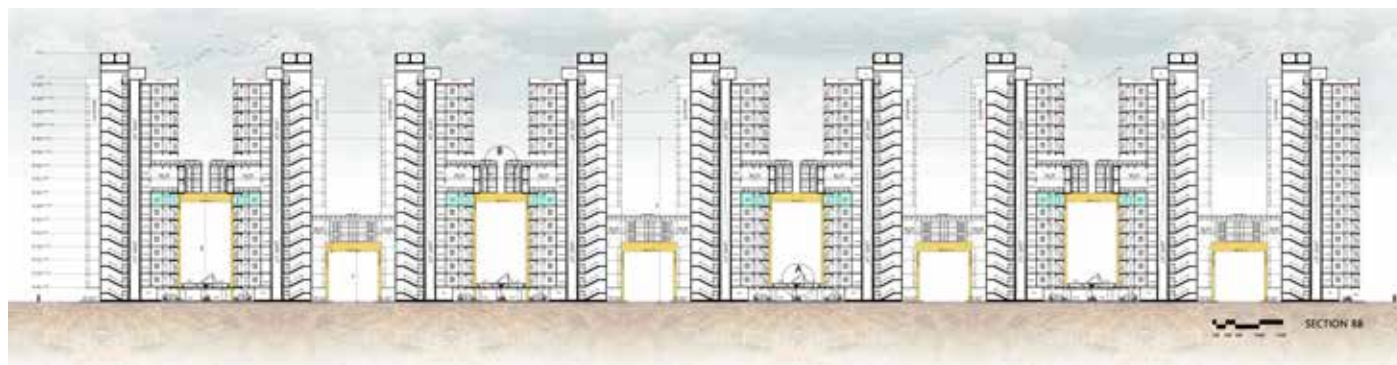
Fig. 9: Section through the middle level connecting bridge and highlighting the double height common space
